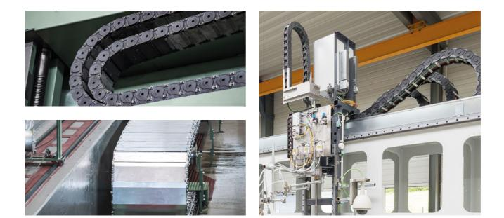
Drag chain systems are used for a wide range of applications and travel distances. EKD Systems has the right solution for every application: from self-supporting drag chains for short distances to gliding drag chains for longer distances. Our range also includes special slide shoes to reduce wear and channel systems to guide the chains. Even for very long movement distances and high additional loads, the Marathon system is a reliable solution.
